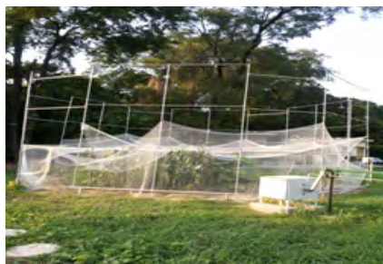
Fig. 3. FACE system at NBRI, Lucknow to determine and control of CO 2 level/concentration in each ring on real time basis.
