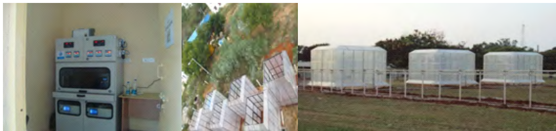
Fig. 1 Open Top Chamber with instrumentation
